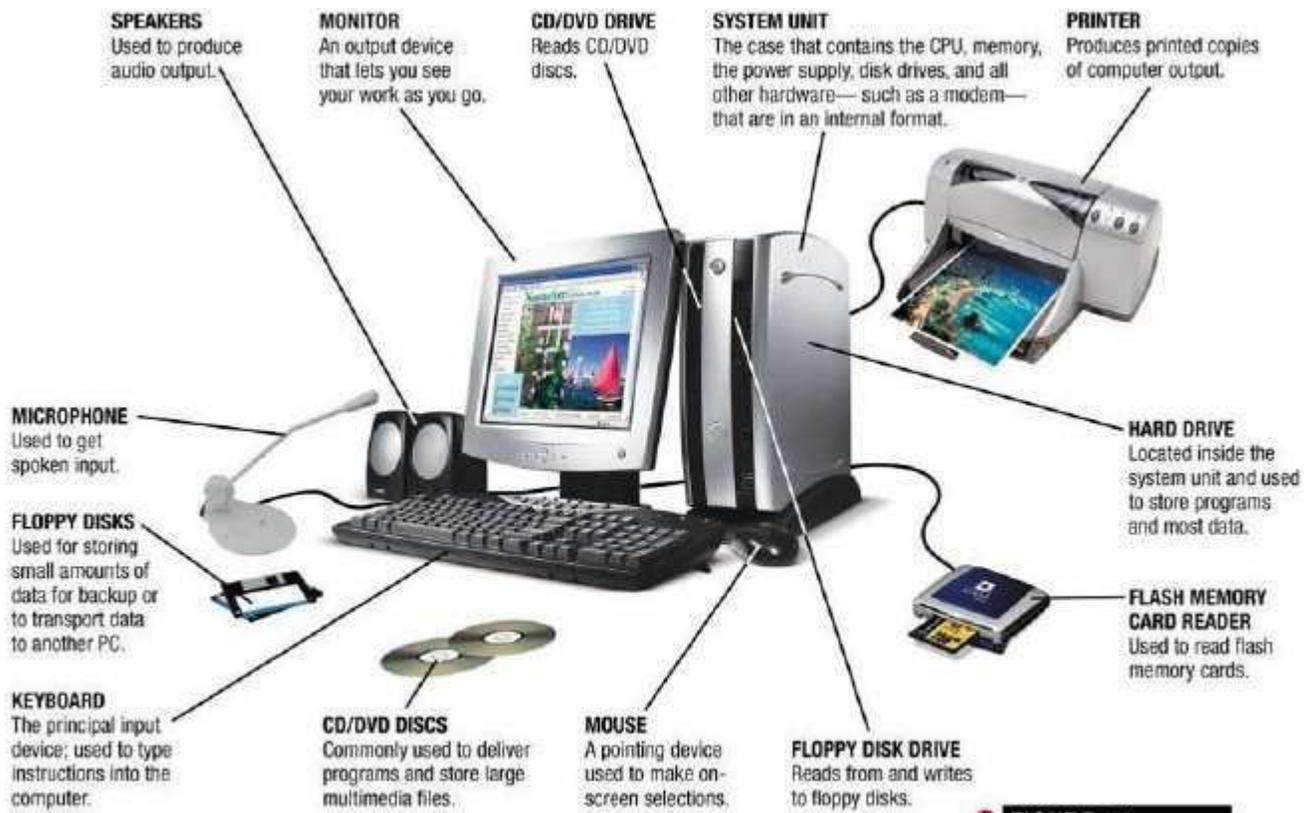
Input and Output device and Storage devices of a Computer:
